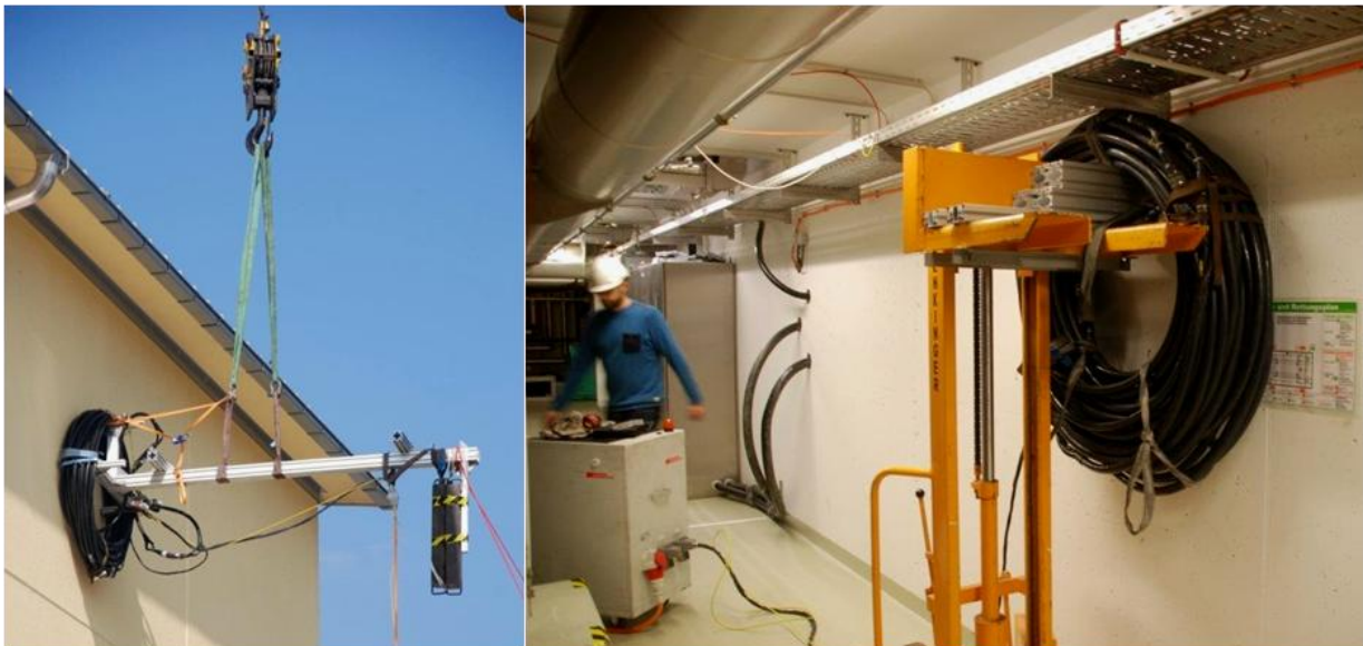
Pulse demagnetization of the KATRIN hall (30x20x15m) with the mobile power module MM DM200-PC and flexible demagnetization cables K8/10-30. The two teams required about 20 hours for demagnetization of the critical areas.
