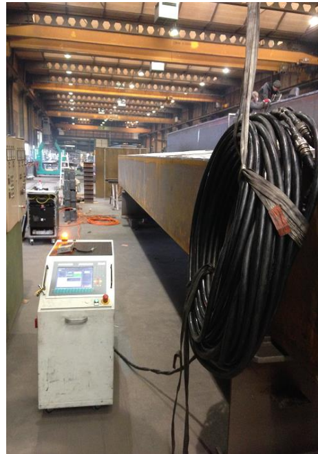
Demagnetization of a steel box girder
